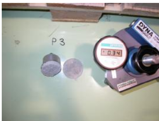
Slike 5, 6 i 7. Rezultat pull-off testa na mernim mestima P1, P2 i P3 Figures 5, 6 and 7. The pull-off test results on measuring points P1, P2 and P3
